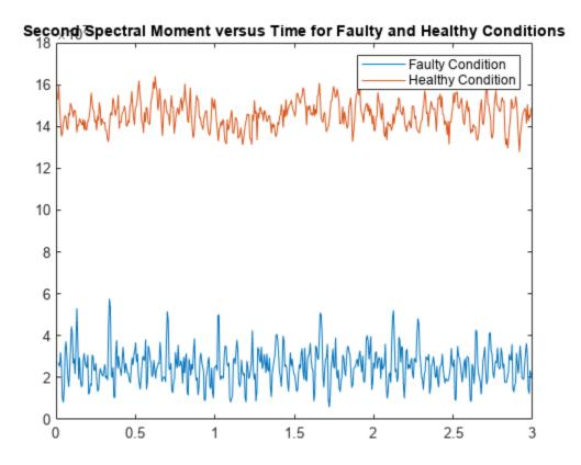
The moment plot shows behavior different from the earlier vibration plot. The vibration data for the faulty case is much noisier with higher-magnitude spikes than for the healthy case, although both appear to be zero mean. However, the spectral variance (second spectral moment) is significantly lower for the faulty case. The moment of the faulty case is still more noisy than the healthy case.
